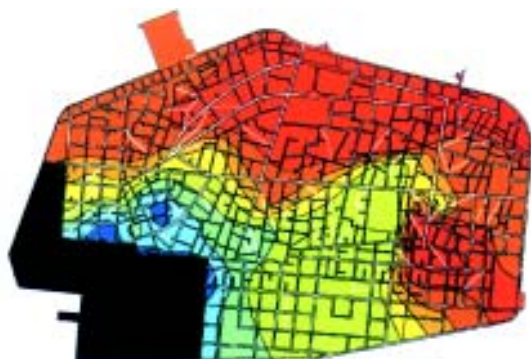
Map 3.1a: Map showing areas that would be inundated in 2025 (high) scenario. That is 0.84m (19.7cm + 64cm*). The same map also applicable to year 2050 (low) scenario. That is 0.84m (19.9cm + 64cm)
