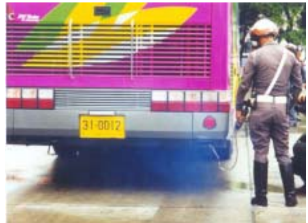
Figure 9.3 Black Smoke Inspection
